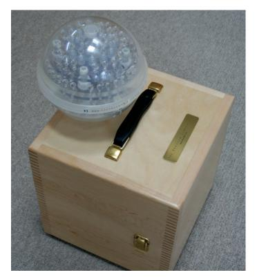
The phantom is supplied with a maple storage case. The case is machined on top to hold the top hemisphere of the phantom if disassembly is required.
