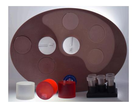
The Liver Phantom combines the advantages of objective test objects and anthropomorphic elements for evaluation of advanced iterative processing.
