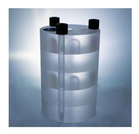
With the automated Smári analysis, Corgi provides an efficient method to measure image quality and dose in cone beam CT systems.
