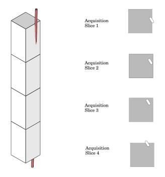
Ilustration of 4 slices with voxels on the left and pixel view on the right. In slice 2 and 3 the wire is within the pixel and on slices 1 and 4 it is also in neighboring pixels.
