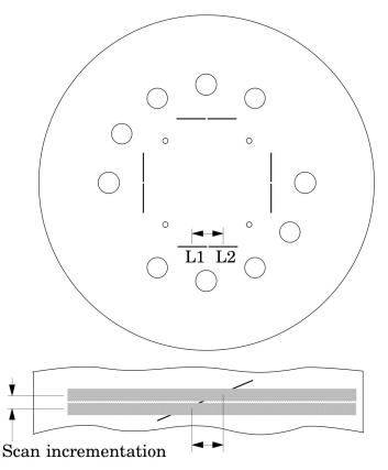
Schematic illustration of two sequential 5mm scans superimposed. L1 is the center point on the  $23^{\circ}$  ramp in the first scan image and L2 is the center point on the  $23^{\circ}$  ramp on the second image.
