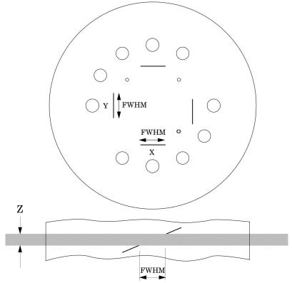
The 23° wire ramp angle is chosen to improve measurement precision through the trigonometric enlargement of 2.38 in the x-y image plane.
