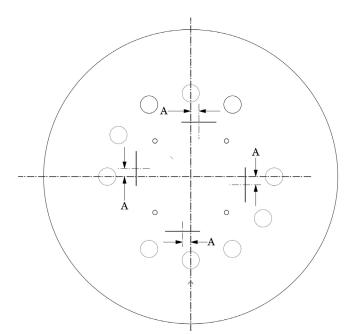
For measuring the z axis alignment lights, measure from the center of the ramp image to the part of the ramp which aligns with the center of the phantom and sensitometry samples. Multiply the distance A by 0.42 to determine the z axis alignment light accuracy. To evaluate x and y accuracy, measure from the center of the phantom to the center of the scan field by use of the grid function or knowledge of the central pixel location.
