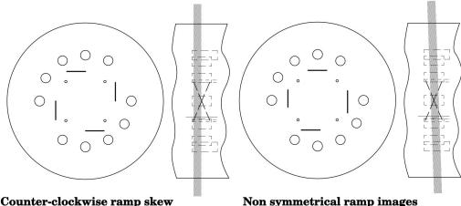
When the ramps are evenly rotated counter-clockwise from center, the phantom needs to be moved toward the gantry.
