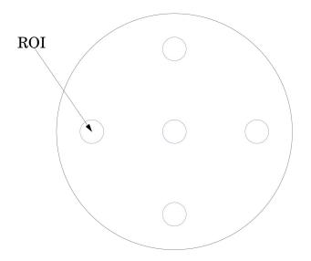
The mean CT number and standard deviation of a large number of points, (say 1000 for example) in a given ROI of the scan, is determined for central and peripheral locations within the scan image for each type of scanning protocol. Inspect the data for changes from previous scans and for correlation between neighboring slices.
