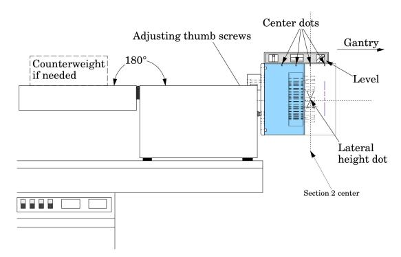
A localizer scan image will show the crossed slice width wires at the z axis center of section 2. By viewing an axial image from the center of Section 2 proper alignment can be verified; see **Phantom position verification** section.
