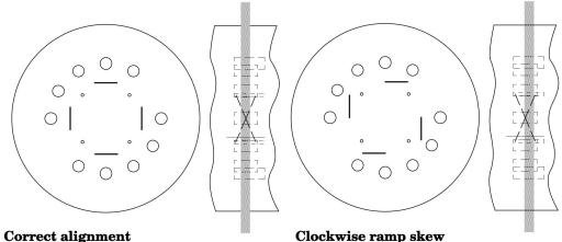
In this image the x, y symmetry of the centered ramp images indicates proper phantom alignment.
