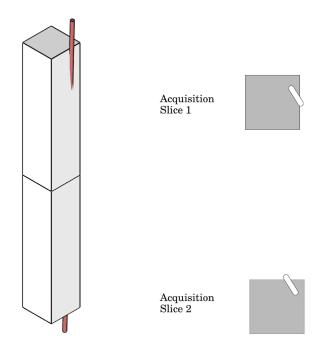
Ilustration of 2 thicker slices on the left and pixel view on the right. In these thicker slices the wire is not contained within any of the pixels.
