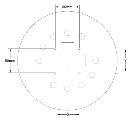
Measuring spatial linearity in x and y axes.
