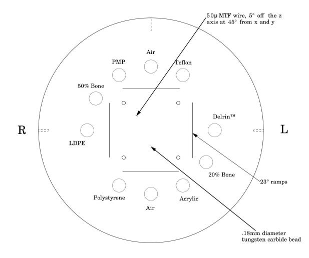
Scan section 2 with slice width, sensitometry, pixel size, MTF bead, and angled wire point source
