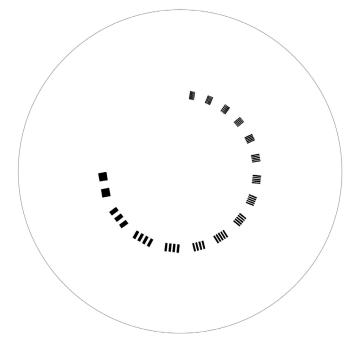
This section has a 1 through 15 line pair per centimeter high resolution test gauge.
