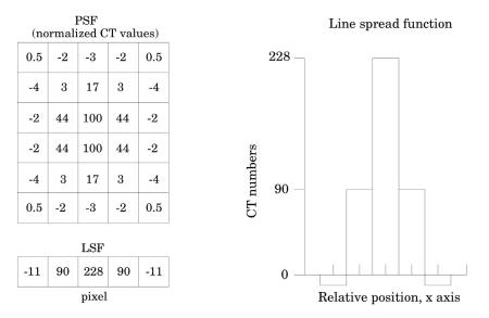
The above illustration shows how by summing the columns (y axis) of numbers in the point spread function (PSF) the line spread function (LSF) for the x axis is obtained.
