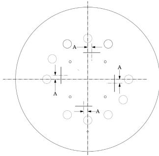
For measuring the z axis alignment lights, measure from the center of the ramp image to the part of the ramp which aligns with the center of the phantom and sensitometry samples. Multiply the distance A by 0.42 to determine the z axis alignment light accuracy. To evaluate x and y accuracy, measure from the center of the phantom to the center of the scan field by use of the grid function or knowledge of the central pixel location.
