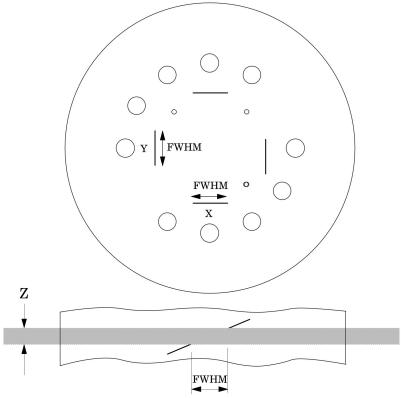
The 23° wire ramp angle is chosen to improve measurement precision through the trigonometric enlargement of 2.38 in the x-y image plane.
