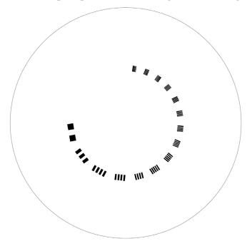
This section has a 1 through 15 line pair per centimeter high resolution test gauge.
