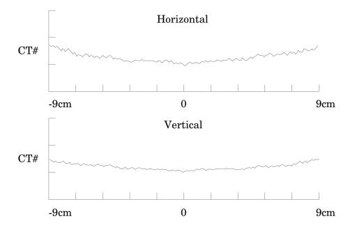
Measure spatial uniformity by scanning the uniformity section. Observe the trends above and below the central mean value of a CT number profile for one or several rows or columns of pixels as shown above.
