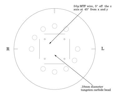
The impulse sources (.18mm bead or  $5^{\circ}$  angled 50 micron wire) are used to measure the point source response function of the CT system.
