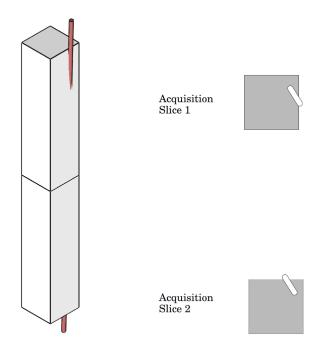
Ilustration of 2 thicker slices on the left and pixel view on the right. In these thicker slices the wire is not contained within any of the pixels.
