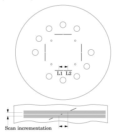
Schematic illustration of two sequential 5mm scans superimposed. L1 is the center point on the 23° ramp in the first scan image and L2 is the center point on the 23° ramp on the second image.
