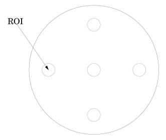
The mean CT number and standard deviation of a large number of points, (say 1000 for example) in a given ROI of the scan, is determined for central and peripheral locations within the scan image for each type of scanning protocol. Inspect the data for changes from previous scans and for correlation between neighboring slices.
