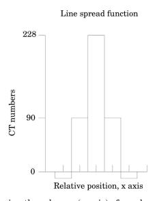
The above illustration shows how by summing the columns (y axis) of numbers in the point spread function (PSF) the line spread function (LSF) for the x axis is obtained.
