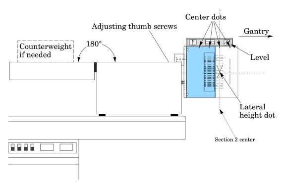
A localizer scan image will show the crossed slice width wires at the z axis center of section 2. By viewing an axial image from the center of Section 2 proper alignment can be verified; see **Phantom position verification** section.
