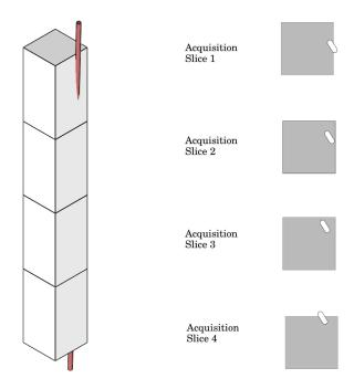
Illustration of 4 slices with voxels on the left and pixel view on the right. In slice 2 and 3 the wire is within the pixel and on slices 1 and 4 it is also in neighboring pixels.
