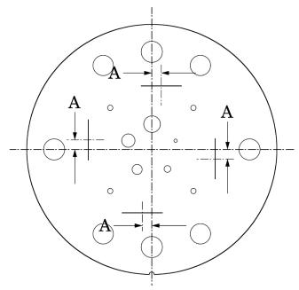
For measuring the z axis alignment accuracy, measure from the center of the ramp image to the part of the ramp which aligns with the center of the phantom and sensitometry samples. Multiply the distance A by 0.42 to determine the z axis alignment light accuracy. To evaluate x and y accuracy, measure from the center of the phantom to the center of the scan field by use of the grid function or knowledge of the central pixel location.
