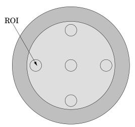
The mean CT number and standard deviation of a large number of points, (say 1000 for example) in a given ROI of the scan, is determined for central and peripheral locations within the scan image for each type of scanning protocol. Inspect the data for changes from previous scans and for correlation between neighboring slices.
