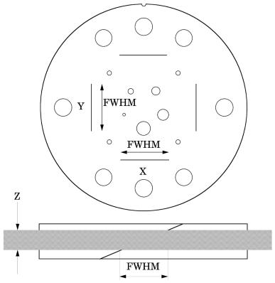
The 23° wire ramp angle is chosen to improve measurement precision through the trigonometric enlargement of 2.38 in the x-y image plane.
