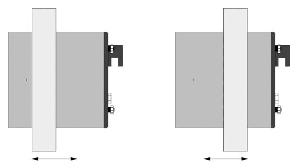
The following optional annuli are designed to be used with the standard 20cm Catphan® housing.
