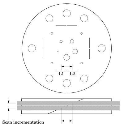
Schematic illustration of two sequential 5mm scans superimposed. L1 is the center point on the 23° ramp in the first scan image and L2 is the center point on the 23° ramp on the second image.
