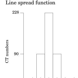
The above illustration shows how by summing the columns (y axis) of numbers in the point spread function (PSF) the line spread function (LSF) for the x axis is obtained.
