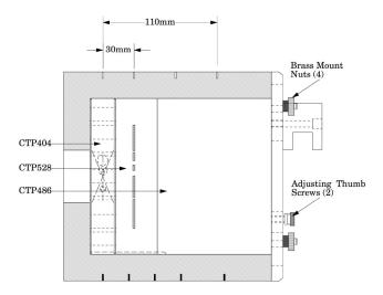
This section has a 1 through 21 line pair per centimeter high resolution test gauge and two impulse sources (beads) which are cast into a uniform material. The beads are positioned along the y axis 20mm above or below the phantom's center and 2.5 and 10mm past the center of the gauge in the z direction. On older CTP528 modules the bead is aligned in the z axis with the gauge.
