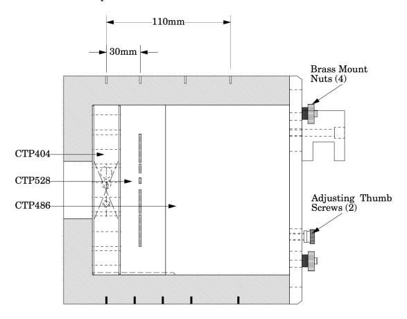
Note: The brass mount nuts hold the mount to the phantom housing. Only the black adjusting thumb screws should be used to level the phantom.
