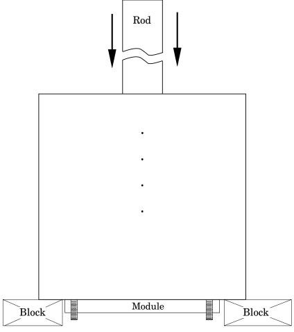
To insert modules hold the phantom housing on its side with the interior alignment key at the top. Align the module notches with the housing key as the modules are inserted one at a time into the housing. The illustrations on page 5 will indicate the correct locations of the modules.
