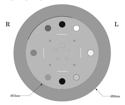
The drawings in this product guide show a schematic view of the modules as they would be seen in a typical head first CT scan where the right side of the phantom is shown on the left side of the image.
