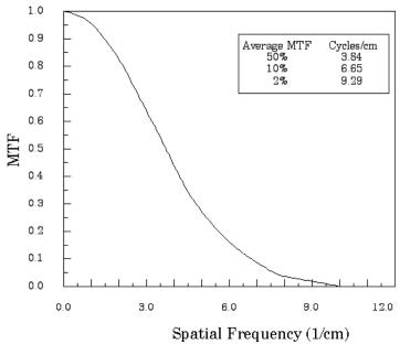
The MTF curve results from the Fourier transform of the LSF data. Generally it is easiest to use automated software for this operation. Some CT scanners are supplied with software which can calculate the MTF from the Catphan® bead images. Independent software is listed in the **Current automated programs available** section of the manual.
