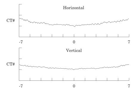
Measure spatial uniformity by scanning the uniformity section. Observe the trends above and below the central mean value of a CT number profile for one or several rows or columns of pixels as shown above.
